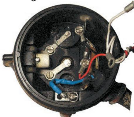
Next, the negative (black) wire from the Bisun needs to be connected either to 'B-' (or its neighbour) or to the '0V' point in the headset, as in the image here. Again, check that this connection does not result in any accidental connection with other parts of the headset.
