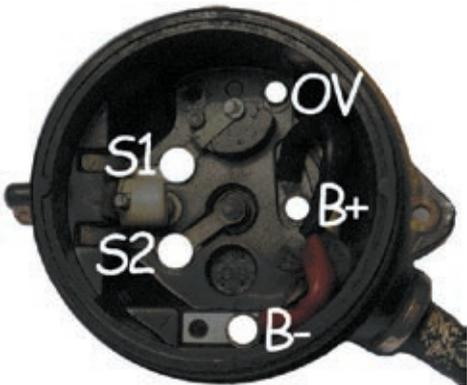
The Bisun requires the switch to be on the positive side of the circuit, hence the positive supply from the battery must be connected to the headset connection labelled 'B+' in the diagram to the left.
