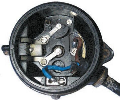
In this image, the sleeving has been removed, and the wires swapped so that the positive (brown) wire is connected to the 'B+' point, and the negative wire to the 'B-' point.
