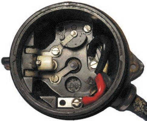
The headset should now contain the two switch contacts, each held down by its own screw, and the two power input leads, and look something like the image on the left.
