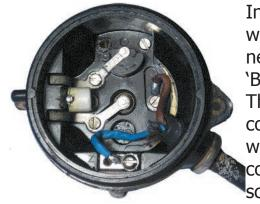
In this image, the sleeving has been removed, and the wires swapped so that the positive (brown) wire is connected to the 'B+' point, and the negative wire to the 'B-' point.
