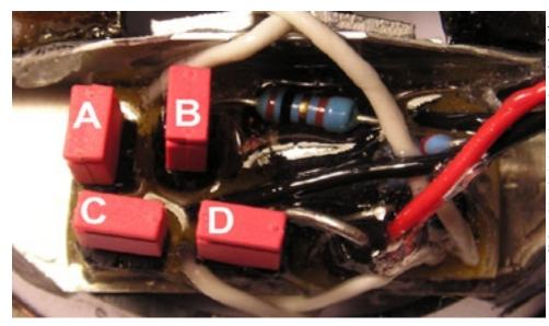
All configuration is done with the headset open, by adding or removing 'jumpers' on the circuit board on the back of the reflector.
