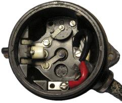
The headset should now contain the two switch contacts, each held down by its own screw, and the two power input leads, and look something like the image on the left.
